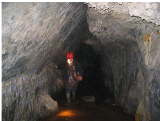
Following the level, the slate vein is clearly visible on the left.
